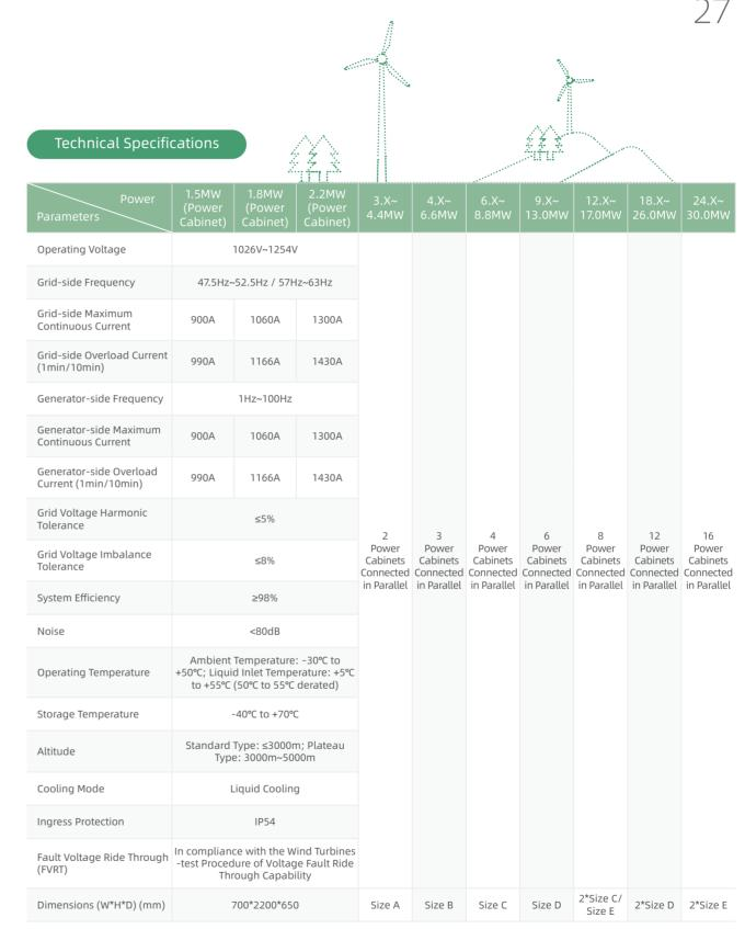
Hopewind power cabinets, distribution cabinets, and liquid cooling cabinets used in the low-voltage three-level full-power converter are all designed with standardized dimensions, allowing flexible layout combinations between cabinets.
