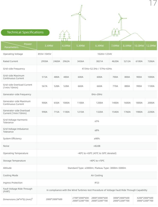
① For dimensions of the doubly-fed converter with the medium-voltage stator, consult Hopewind.
